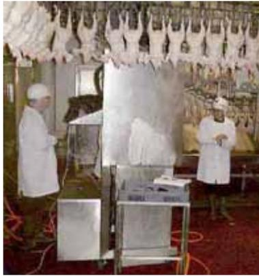
A pilot scale atmospheric steam cabinet has been developed and successfully used in many experimental trials involving poultry, pork, lamb, and beef (and also fish, fruits and vegetables) both in a laboratory setting and alongside commercial processing lines in industry to demonstrate the effectiveness of steam interventions in lowering microbial loads.
