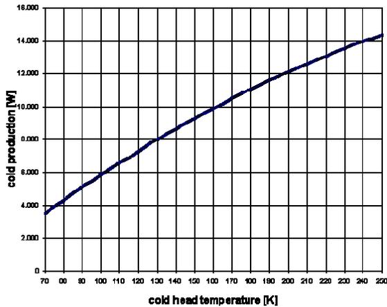
**Figure 4.4** Cooling capacity of SPC-4 Stirling process cryogenerator vs cold head temperature (*Stirling Cryogenics & Refrigeration BV*)
