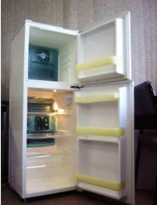
**Figure 5.10** 126 litre thermoelectric refrigerator/freezer prototype (from Davis et al, 2004)
