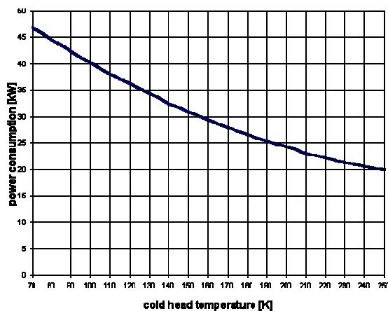
**Figure 4.5** Power consumed by SPC-4 Stirling process cryogenerator vs cold head temperature (Stirling Cryogenics & Refrigeration BV)
