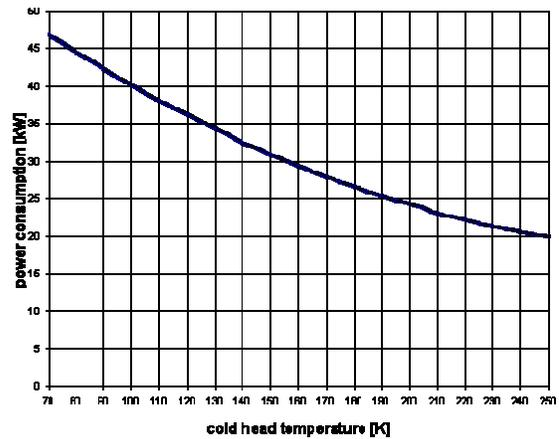
**Figure 4.5** Power consumed by SPC-4 Stirling process cryogenerator vs cold head temperature (*Stirling Cryogenics & Refrigeration BV*)
