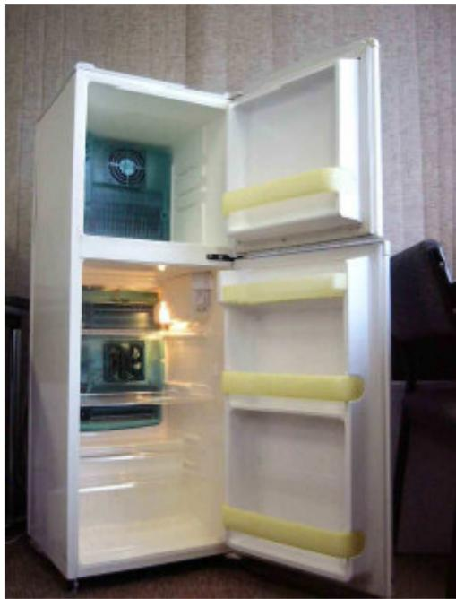
**Figure 5.10** 126 litre thermoelectric refrigerator/freezer prototype
