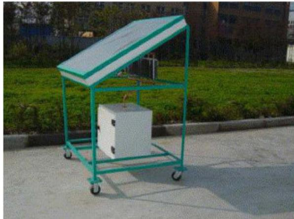
**Figure 1.20., No Valve Solar Adsorption Ice Maker:** (1) Cover Plate, (2) Adsorbent Bed, (3) Insulation Material, (4) Ice Frame, (5) Condenser, (6) Connecting Pipe, (7) Evaporator, (8) Water Tank, (9) Insulation Box.
