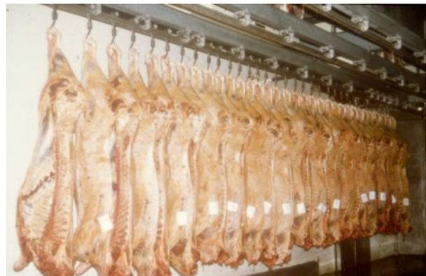
Data were from 14 commercial beef chilling that ranged in capacity from 18000 to 93000 kg (mean 30625 kg) of beef in carcass form and in size from 216 to 1124 m<sup>3</sup>. The energy data was broken down into a base demand and a product demand (see table 1). Base demand is
