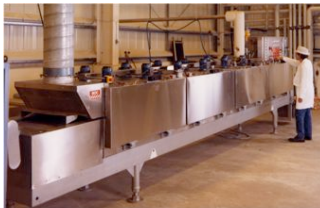
Nitrogen tunnel freezer
